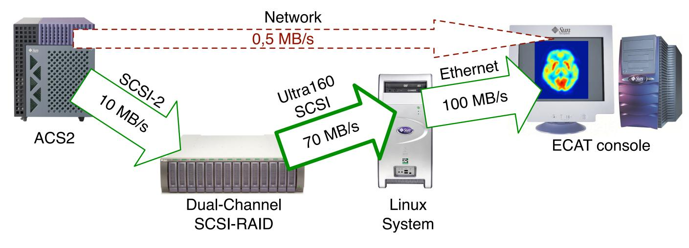
The ACS2 uses a standard SCSI-2 hard disk for storing the raw acquisition data and allows to transfer data to other systems with a throughput of  $\approx$  0.5 MB/s only. We replaced the internal hard disk with an external dual-channel SCSI-RAID system and connected one channel to the ACS2 and the second to a separate Linux system. To access the data from the Linux system, we reverse-engineered the file-system used by the ACS2 and developed an own implementation for the Linux operating system.
