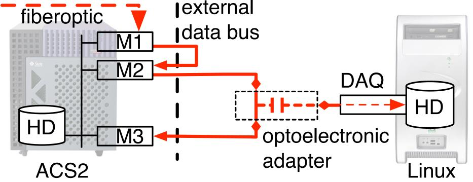
The raw coincidence data during a PET acquisition is routed through externally accessible data cables in the ACS2 system. This data bus consists of 32 channels and connects all main acquisition components (M1-M3) of the ACS2 while carrying the typical list-mode data
