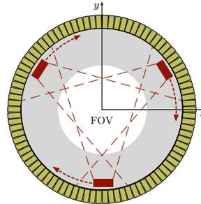
**Fig. 1.** Schematic view of the three rotating radioactive transmission sources  $^{68}\text{Ge}$  located in an ECAT Exact HR<sup>+</sup> PET scanner.
