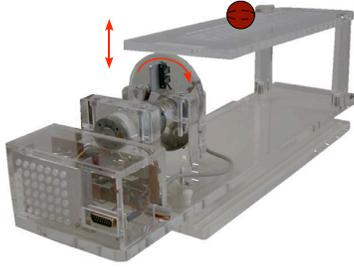
**Fig. 2.** Respiratory motion phantom [6] with motion tracked steel ball attached (red sphere).
