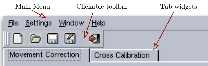
Figure A.2: The application window of lmmc has three main components. A main application menu, a click-able toolbar and two tab widgets for either the movement correction or cross calibration.
